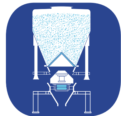
1. Bin lowered onto discharge station.
